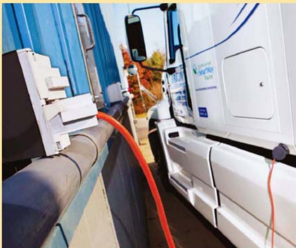
A Braun's Express truck is hooked up to an electric outlet at the carrier's facility. The carrier says the reduction in idling provides significant savings.
